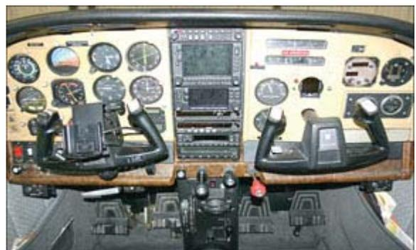
**Bill Hunt's panel, upgraded in 2003 with Garmin GNS530/430 GPS, a GTX 330 transponder and audio panel, Bendix/King ADF, an HSI, flight director system, RMI and STEC-55 autopilot.**
